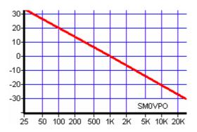
To correct this state of affairs, the record player must have an equal and opposite curve. A simple RC time-constant will give the required slope, but not over a full 60dB range. Two time-constants are commonly used so that as one "flattens off" so the other one comes into action. This I did using negative feedback in a simple Op-Amp circuit. The target response is shown to the side of this text.
